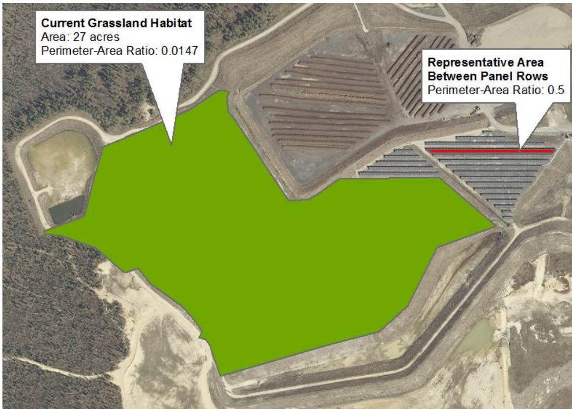
Figure 3. Current grassland habitat area and representative area remaining between solar panel rows for comparison of perimeter-area ratios. The representative area is typical of what would be left as suitable grassed areas between panels across the Diversion Area.
