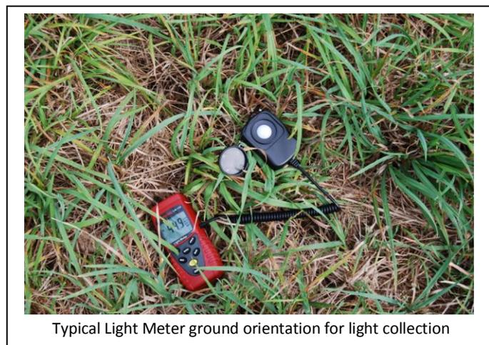
A series of light recordings were collected to estimate the survival and final disposition of the current landfill grasses. The readings were collected in various grass dominated conditions, existing solar panel arrays as well as under a simple shade test assembly.
